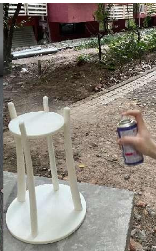
Figure 25. Product Grinding and Spray-Painting Process (Designed and Photographed by the Author).
