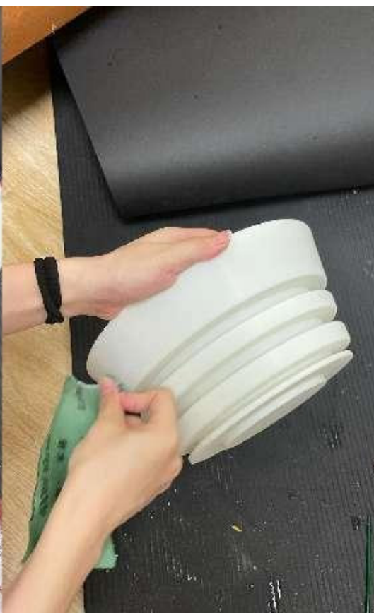
Figure 25. Product Grinding and Spray-Painting Process (Designed and Photographed by the Author).
